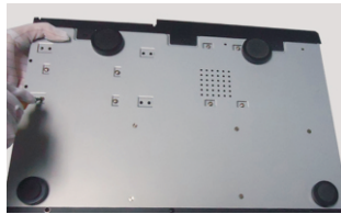
④ Turn over the machine and secure the HDD with the screws.
