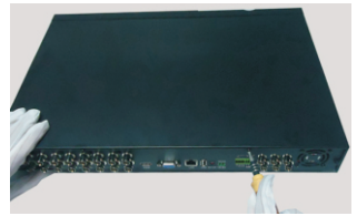
⑥ Install back the cover and secure it with the screws.
