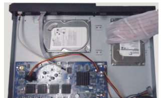
③ Put the HDD onto the bottom of the machine.
