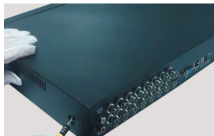
② Loosen the screws on the side to open the cover.
